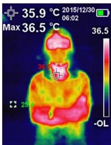
Center point marking and full-screen automatic tracking of high and low temperature, while displaying temperature
