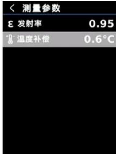
Self-adjusting emissivity and responding to temperature compensation and correction in different environments and places
