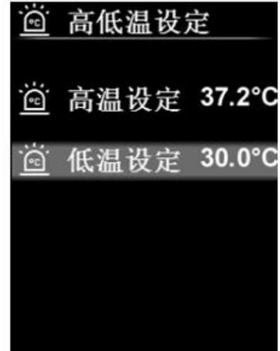
The temperature limit function of high temperature alarm and low temperature alarm can be set according to the actual application scenario
