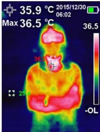
Center point marking and full-screen automatic tracking of high and low temperature, while displaying temperature
